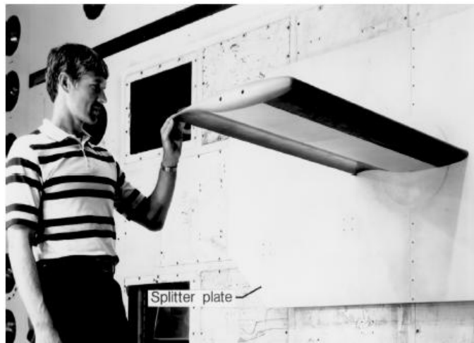
Figure 1: Rectangular Supercritical Wing mounted in the NASA Langley Transonic Dynamics Tunnel.
