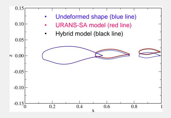
The final deformation of the wing is about 1% displacement in the wingnormal direction and 0.4 degrees twist measured at the wing tip.
