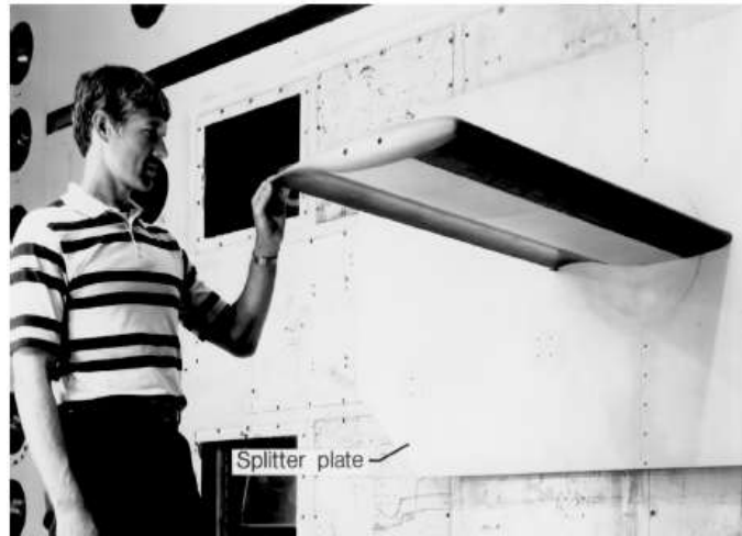
Figure 2: Rectangular Supercritical Wing mounted in the NASA Langley Transonic Dynamics Tunnel.
