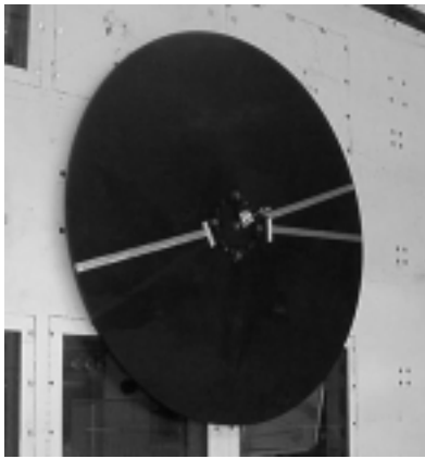
Figure 4: Inertia model used during OTT shakedown testing.
