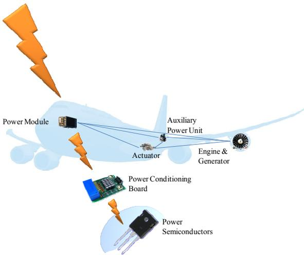
Figure 2. Propagation of lightning event through avionics.
