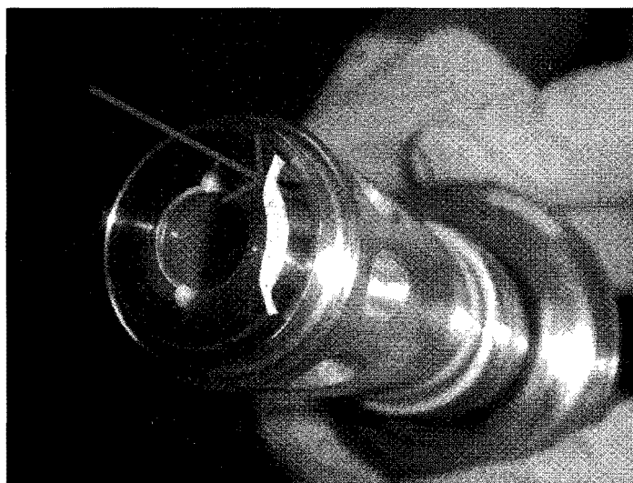
Fig. 2. The arrow indicates where the break occurred in the poppet of the Flow Control Valve on one of the SSMEs during the mission STS-126 of Space Shuttle Endeavor. The break resulted in increased flow of gaseous hydrogen but did not result in an issue during launch
